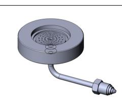
Tighten the screws of the filter supporting base (2) and the outlet connection nozzle (3) with a spanner.
