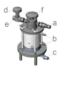
Nozzle a: connected to the female of high-pressure nitrogen connection (12) Joint b: connected to the water bath tubing Joint c: connected to the product tubing d: deflation valve Joint e: gas vent f: feed port
