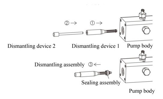
Figure 5 Dismantling of sealing parts
