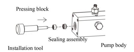
Figure 6 Installation of sealing parts
